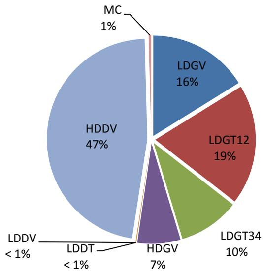
Figure 3 – 2008 On-road NO<sub>x</sub> contributions by vehicle type for the OSO area
